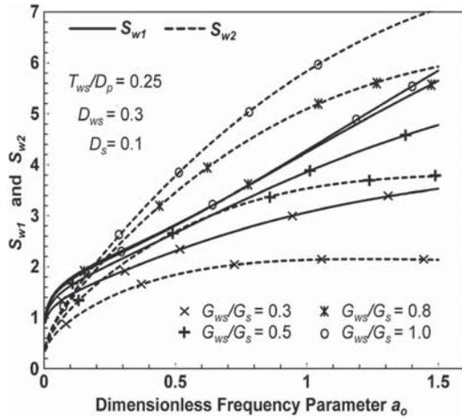
Figure 2. The variation of dimensionless soil stiffness and damping parameters with dimensionless frequency for different shear modulus reduction ratio.
