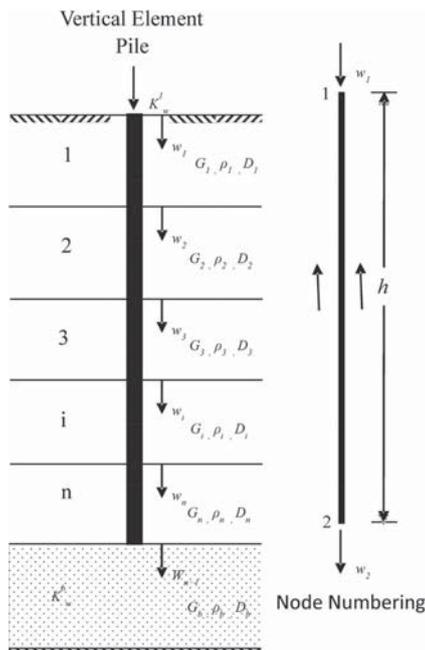
Figure 3. Pile embedded in soil strata with nodes numbering.
