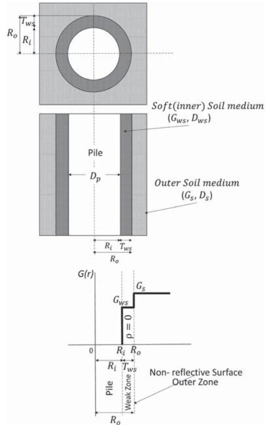
Figure 1. Schematic representation of cylindrical boundary zone around the pile and the variation of shear modulus of soil in the layered soil media.
