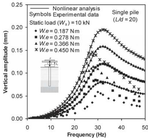
Figure 5. Comparison of experimental and theoretical response of single pile without pile-soil separation.
