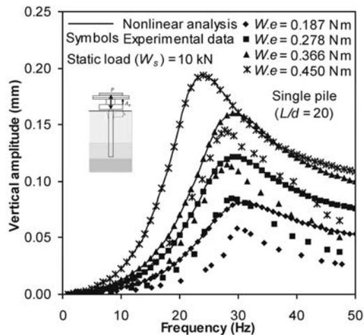
Figure 6. Comparison of experimental and theoretical response of single pile considering pile-soil separation.
