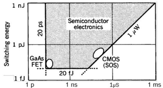
Fig. 2 Limits of switching energy, time, and power of silicon-on-sapphire (SOS) & complementary metal-oxide-semiconductor (CMOS)
