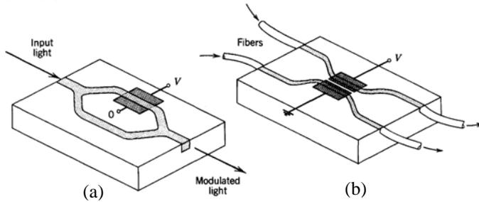
Fig. 4 (a) 1x1 switch Mach-Zehnder interferometer (b) A 2x2 switch using an integrated electro-optic directional coupler.
