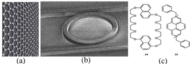
Fig. 10 (a) Graphene (b) By making a ring resonator either transparent or opaque to a particular wavelength of light, a photonic circuit can control it as a tiny photonic switch. (c) Molecular level implementation of XOR gates i by photo induced electron transfer (PET) mechanism.
