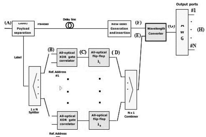
Fig. 8 All-optical packet router architecture.
