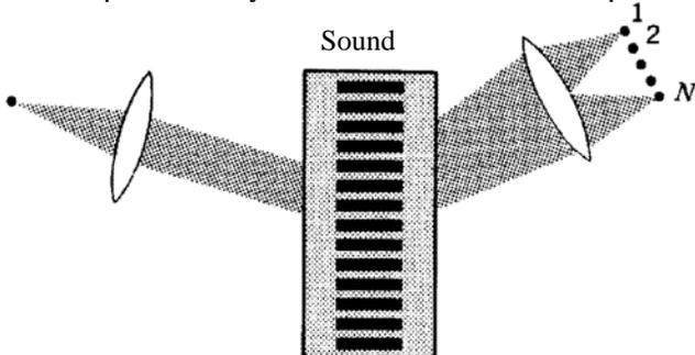
Fig. 5 Acousto-optic switch.
