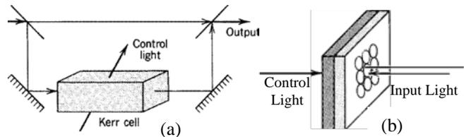
Fig. 7 (a) All-optical 1x1 switch using Mach-Zehnder interferometer exhibiting optical Kerr Effect. (b) An all-optical array of switches using an optically addressed liquid-crystal spatial light modulator.
