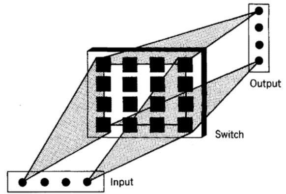
Fig. 6 4x4 magneto-optic crossbar switch. Each of the 16 elements is a 1x1 switch transmitting or blocking light depending on the applied magnetic field.
