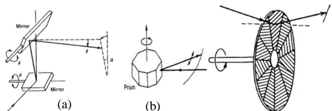
Fig. 3 Deflecting light into different directions using (a) rotating mirrors; (b) a rotating prism; (c) a rotating holographic disk
