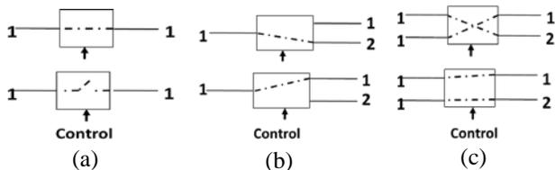
Fig. 1 (a) 1 X 1 switch. It is an on-off switch. (b) 1 x 2 switch connects line to either of two lines. (c) 2 X 2 crossbar switch connectivity
