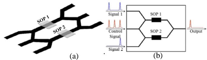
Fig. 9 (a) Mach-Zehnder Interferometer with one SOA in each arm commonly known as SOA-MZI. (b) XOR architecture based on a SOA-MZI. Two SOAs are symmetrically placed in each branch. XOR operation is achieved by XPM in the SOAs.
